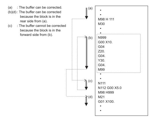
(4) With buffer correction, as EOB (;) in the comment block is treated as a line feed code, when edited and saved with buffer correction, the program error occurs.
