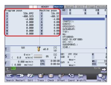
(1) The maximum number of axes that can be displayed is 10 axes. Press the menu [Next axis] to switch display to display the subsequent axes.
