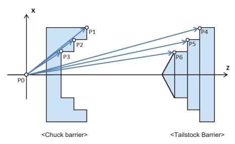
The barrier data which is set on this screen will be set to NC by converting to the parameter "#8301 P1" to "#8306 P6". Specify the workpiece center coordinates (P0) of X axis for the chuck and tailstock in advance with the parameter "#8300 P0" on the menu [Barrier data] of parameter screen. The workpiece center coordinates (P0) of Z axis are the machine coordinates zero point.
