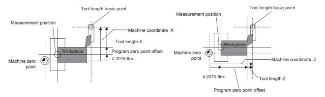
The tool length is automatically calculated by the following formula:
