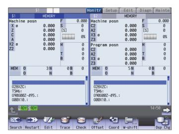
(1) The maximum number of axes that can be displayed is 8 axes. Press the menu [Next axis] to switch display to display the subsequent axes.
