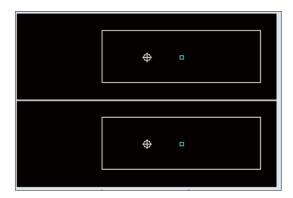
The white-framed display range in the upper and lower areas simultaneously move to the left/right when the  $[\leftarrow]$ ,  $[\rightarrow]$  keys are pressed.
