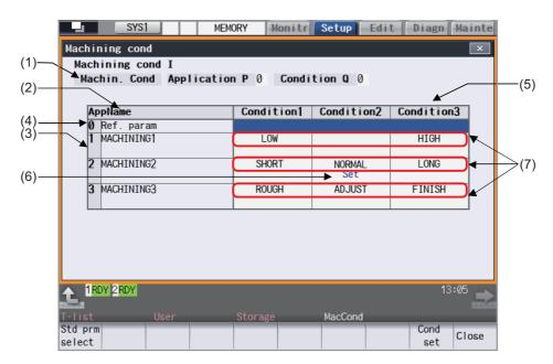
When the parameter "1760 cfgPR10/bit0" is set to "1".
