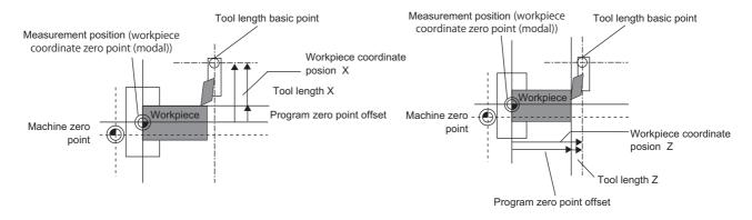
The tool length is automatically calculated by the following formula:
