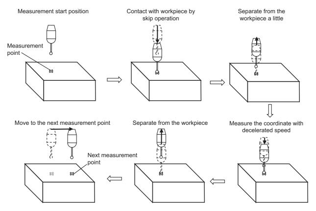
The measurement is started from the position one third away from each side in the direction perpendicular to the measurement face for each measurement point.
