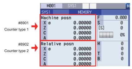
■[Quad counter](2-part/3-part system simultaneous display)
