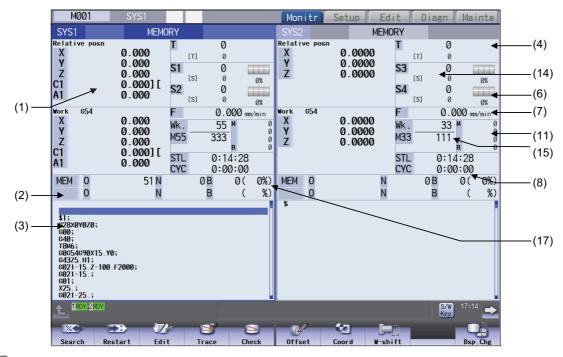
(1) The maximum number of axes that can be displayed is 5 axes. Press the menu [Next axis] to switch display to display the subsequent axes.
