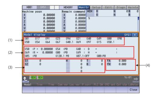
Even if operating area is switched in the 2-part system simultaneous display, the position of the pop-up window will not change. It is always displayed at the bottom of the screen.
