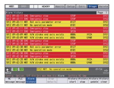
When an alarm occurs, the alarm information is recorded. When the NC power is ON, an alarm is automatically recorded in alarm history. Alarm information is recorded from the latest alarm to 512.
