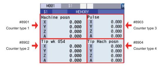
■[Quad counter] (4-part system simultaneous display)
