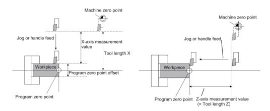
The tool length is automatically calculated by the following formula: Tool length = Measurement position - Program zero point offset (L)
