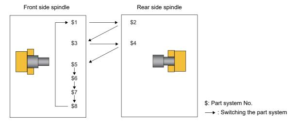
When the rear side spindle exists, and operation is started with the 2nd or 4th part system, the workpiece is assumed to be mounted to the rear side spindle.
